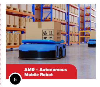
Self-operated robots designed to move materials guided by sensors, lasers, or radar, similarly to how a robotic vacuum cleaner operates. Can detect and avoid obstacles, and move freely around the warehouse floor. Typically used for zone picking and replenishing to create collaborative workflows with human workers.
