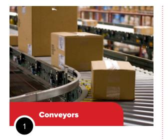
Fixed machinery that automatically moves items from point A to point B on a moving belt or rollers.
