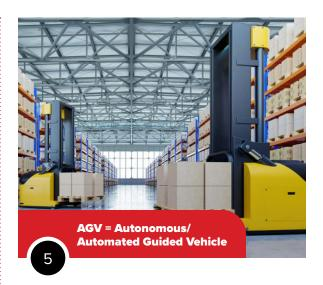
Vehicle that moves materials or people along predetermined routes guided by physical aids, like lasers, cameras, wires or magnets. Comes in many forms, including with or without human interaction, and safety features like collision avoidance. Best used for repetitive tasks of moving things from point A to point B.
