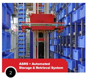
Fixed machinery featuring automated picking that delivers items to an end-point, similarly to how a vending machine functions. Works best in predictable environments with uniform picking patterns.
