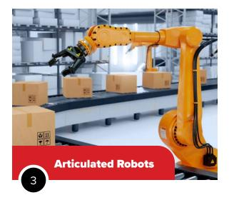
Robots with multiple rotary joints, often designed to mimic human arm movement. Primarily used for simple, repetitive tasks, including picking, palletizing, sorting, receiving and replenishing. Humanoid robots are the next-generation, advanced version of articulated robots, but are mostly still in development and not widely available.
